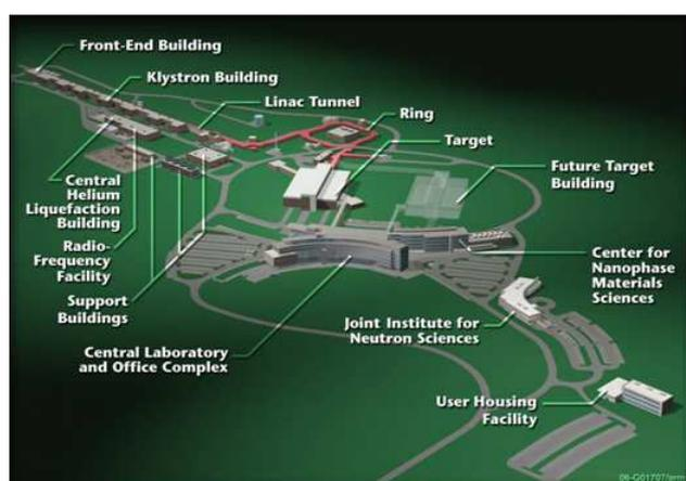
Figure 1. Layout of the Spallation Neutron Source
