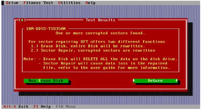
If the test should fail and the cause of failure is due to a media error (for example a bad write) then you will be presented with a screen similar to that shown below.
