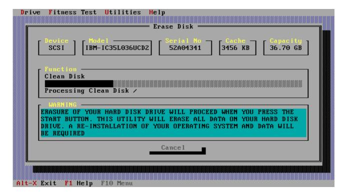
After completing the erasure of the disk a sequential read of the disk is carried out to verify that all sectors have been initialised.
