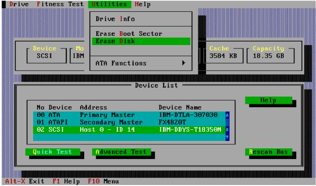
This utility will write zeroes to every sector of your hard drive including the boot sector, and can be used with both IDE and SCSI drives. This utility is meant to be used to clean-up disk which have errors written to the media (e.g. where a system has been powered off whilst writing data out to the drive). This utility can take a long time to run (more than an hour) depending on the capacity of the drive and the system configuration.
