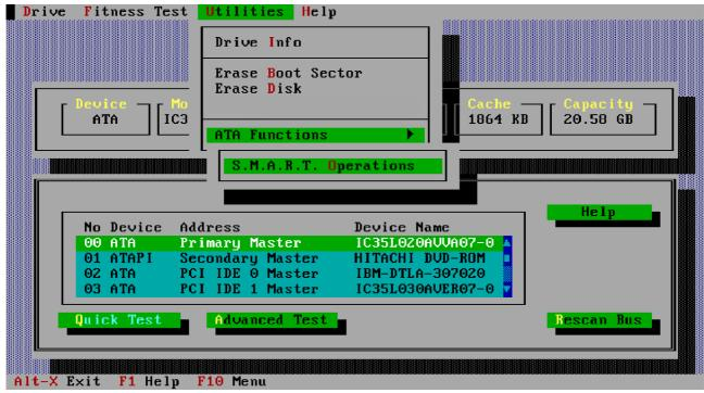
S.M.A.R.T. - Self-Monitoring, Analysis and Reporting Technology is intended to protect user data and prevent unscheduled system downtime that may be caused by predictable degradation and/or fault of the disk device. By monitoring and storing critical performance and calibration parameters, S.M.A.R.T. devices employ sophisticated data analysis algorithms to predict the likelihood of near-term degradation or fault conditions.
