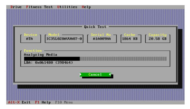
In the screen above, the DFT test is running. The name of the active part of the test is displayed above the progress bar, (in this example - Analysing Media). The progress bar illustrates progress through the active test stage. DFT execution for the Quick Test should be less than 3 minutes in most circumstances
