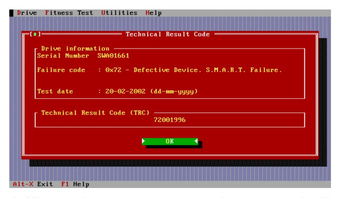
The failing return code 0x72 represents a S.M.A.R.T. error. The S.M.A.R.T. system is a disk drive's way of notifying of possible failure in the future (see Utilities Section of this document for more information on S.M.A.R.T).
