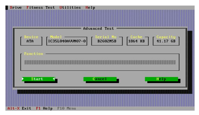
DFT only performs a read test in the user data area, so your data will not be overwritten. Execution time will normally be in the order of 40 minutes, but this can be longer for very large capacity drives. Test progress will be illustrated as shown below.
