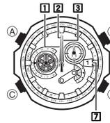
5. After confirming that the **1** Hour Hand and **3** Minute Hand are in their correct home positions, press **C**. This will advance to day home position adjustment.
