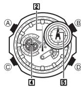
2. After confirming that the **4** Left Dial hand is in the correct home position, press **C**. This will switch to **5** Right Dial Hands home position adjustment.
