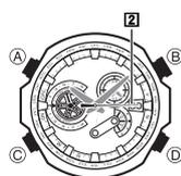
(2) **Second Hand** moves to 3 o'clock, indicating the Home Position Adjustment Mode. See "To adjust home positions".
